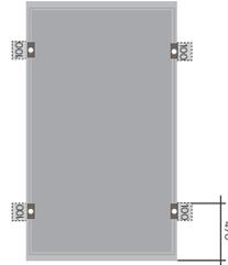
Max. permitted pressure load up to 2,400 Pa (test load 3,600 Pa)
