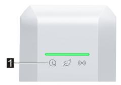
If the charging current is limited by a smart charging current specification, the smart charging symbol lights up. In this case, the charging current limit can be waived once for the current charging session using the touch button (1) (contact surface), if this is permitted by the grid operator. This charges the vehicle faster, if needed.
