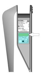
A charging station with an (optional) **calibrated** energy meter has a two-line LCD display on the right side. This display shows the status of the energy meter and additional information.
