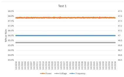
Voltage = 85% of nominal (195.5 V), Frequency = 47.5 Hz, Power Factor = 1,
